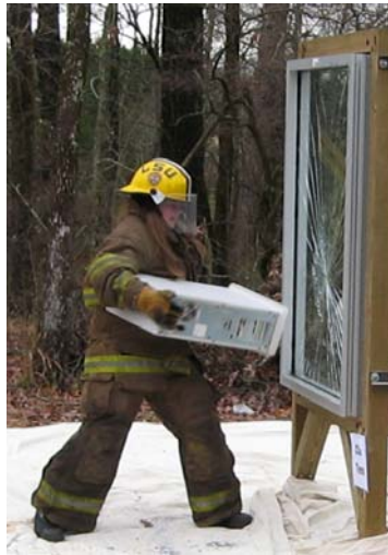
Figure 6. Woman unsuccessfully attempting to pass through a hardened window system by using office furniture (computer) as egress tools.
