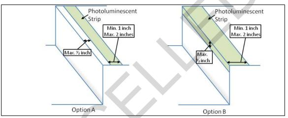
Figure 1: Graphical Representation of Stair Photoluminescent Striping Requirements
