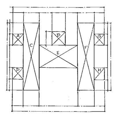
DIAGRAM SHOWING METHOD OF SUBDIVIDING BUILDING FOR GROSS AREA COMPUTATION
