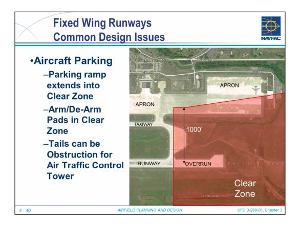
• Aircraft Parking Aprons, especially at old bases, can fall within newer expanded Clear Zone
