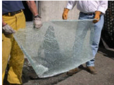
Figure 5: Test 3 Tempered Glass with Daylight Film
