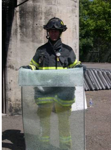
Figure 8: Test 26 Laminated Single Paned Tempered Glass
