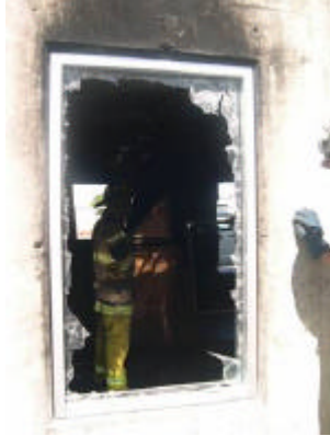
Figure 6: Test 6 Annealed Glass with 4-Sided Attached Film Without Center Seam
