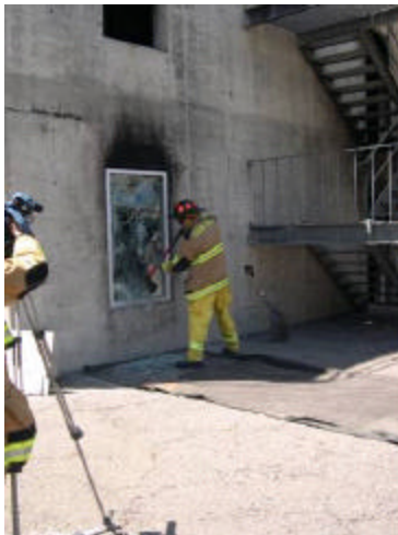
Figure 9: Laminated Annealed Insulating Glass Unit
