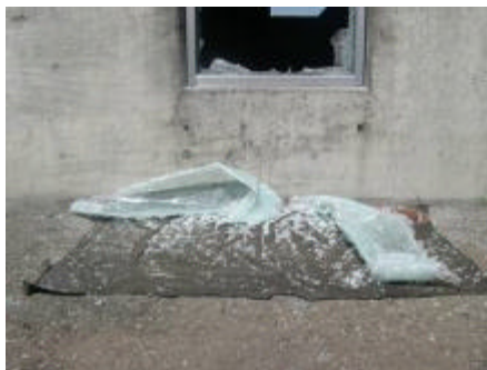
Figure 7: Tempered Glass 4-Sided Attached Film with Center Seam
