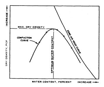
Figure B-1. Compaction curve.
