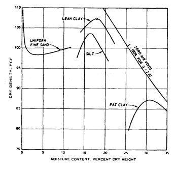
Figure B-2. Typical compaction test curves.
