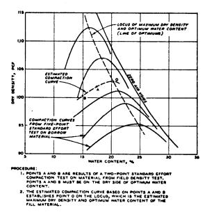
Figure B-6. Illustration of two-point compaction method
