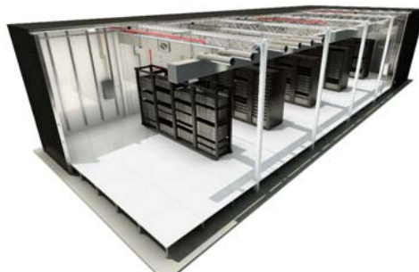
Figure 6 – iFortress pre-engineered data center
