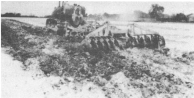
Figure 4-36. Mixing with a disc harrow.
