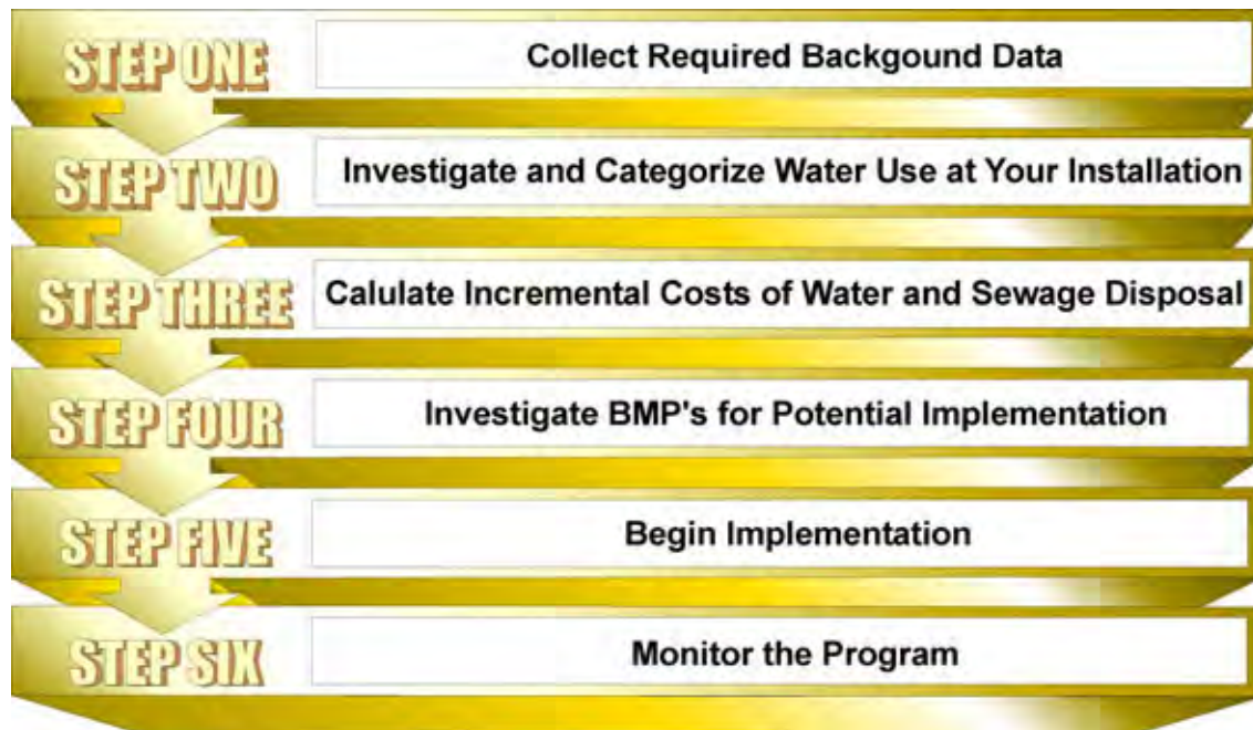
FIGURE 2.1 Six-Step Approach to Water Conservation Plan Development
