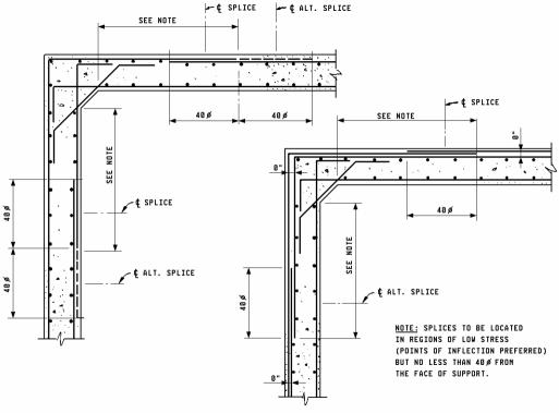
Figure 4-85 Typical horizontal corner details of conventionally reinforced concrete walls
