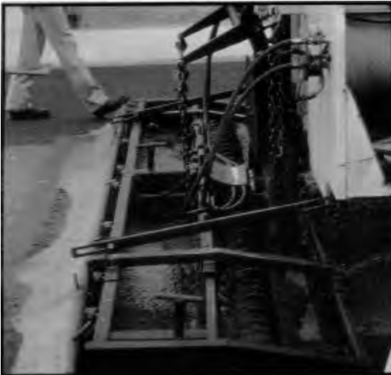
Figure 6.1. View of slurry seal machine
