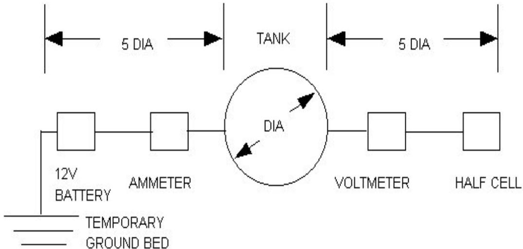
A6.2.1. Install a temporary ground bed of three or four 1.52-meter (5-foot) ground rods at a distance equal to five tank diameters. Place a copper-copper sulfate half cell on the opposite side of the tank. Place it at a distance equal to five tank diameters and along an imaginary straight line through the center of the tank. Make sure it has good contact with earth.
