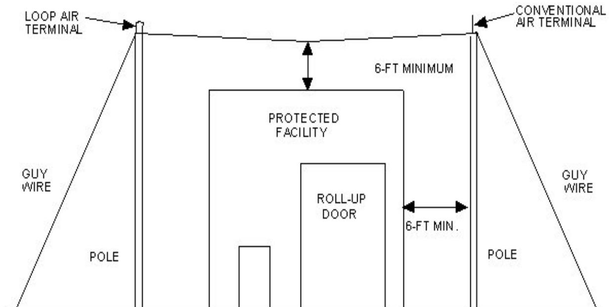
A4.2.3. An air terminal extending above the top of the pole must be securely mounted to the top of the wooden mast and connected to the grounding system. An overhead ground wire or a down conductor, extending above or across the top of the pole, may serve as the air terminal. Each nonmetallic mast must have two down conductors. Metal masts do not require air terminals and down conductors, but must have two connections to the grounding system.
