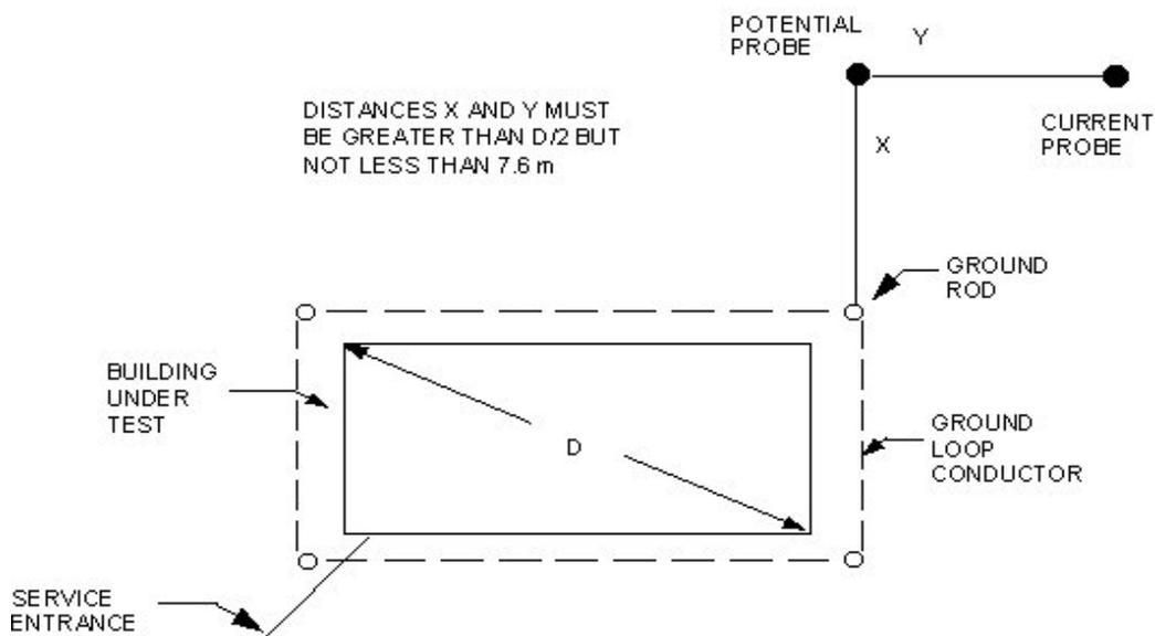
**A6.2. Resistance Test for Above-Ground Petroleum (POL) Tanks.** The method described in paragraph A6.1 is appropriate for medium to small grounding systems. Figure A6.2 illustrates how to measure resistance to earth of larger, more complex systems such as a large POL tank or a substation. In areas where the soil resistivity is relatively high, a higher voltage supply may be necessary. Local cathodic protection technicians can usually furnish the material for the test.
