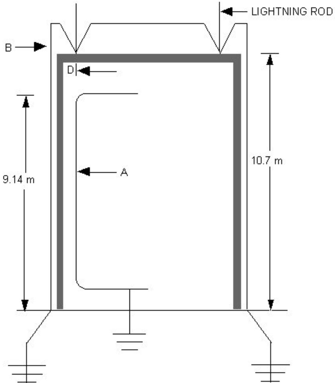
**Figure A3.2. Typical Bonding Conditions in Structures Greater Than 12.2 Meters (40 Feet).**
