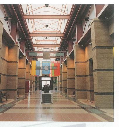
Plain concrete or concrete block walls (painted or unpainted) are not appropriate in non-industrial areas. Use commercial grade wall coverings. Provide noise control and water resistant materials when required. Protect walls and corners in high-use areas. Limit the use of wood paneling to accents and wainscotting.
