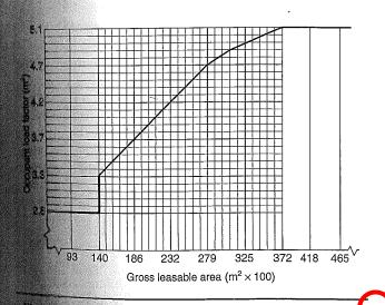
Figure 7.3.1.2(b) Mall Building Occupant Load Factors (M Units).
