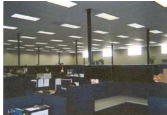
Fig. 14 Newer base building interior illustrating poor quality lighting with high brightness differences and dark furnishings
